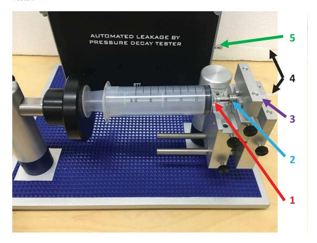
In this example the small-bore connector under test is on the end of a syringe. The volume of space inside the small-bore connector (and syringe) that will be under test (1) must be determined, along with reference connector (2), Festo fitting (3 (sitting out of view behind the grip)), hose (4) and connector (5) to the test equipment.
